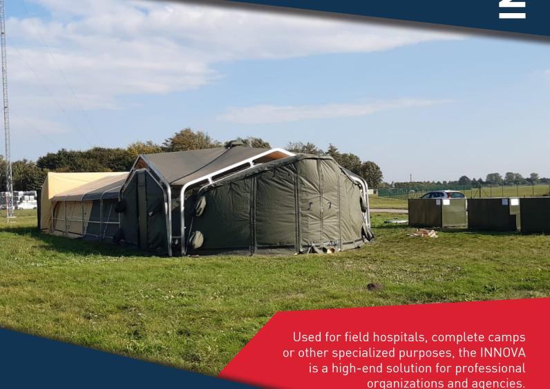
The INNOVA tent is introducing a new type of tent with high comfort by combining simple logistics, high quality, and capability to withstand extreme weather conditions due to tensioned fabrics.
